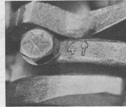
44.12 Identification mark on main bearing cap
