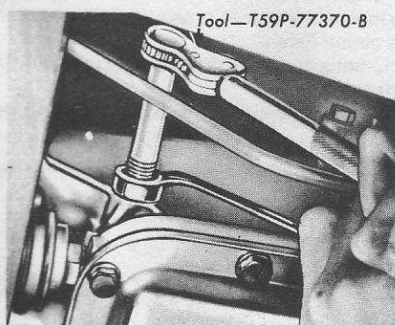
Fig. 6.44 Adjusting low (reverse band) (Sec. 36)
