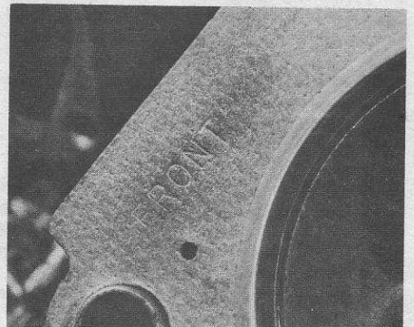
48.8B The word FRONT ensures correct positioning of the cylinder head gaskets
