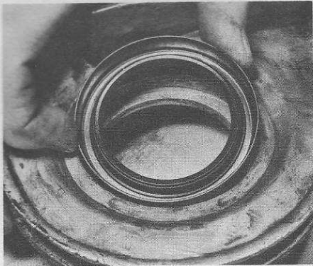
46.8 Installing the timing cover oil seal
