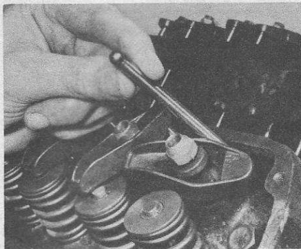
48.11 Inserting the pushrods
