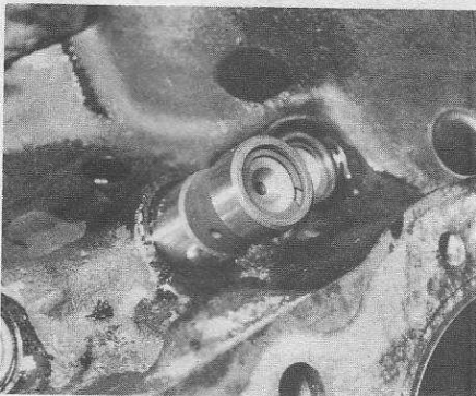
48.7 Inserting a hydraulic valve lifter into the block
