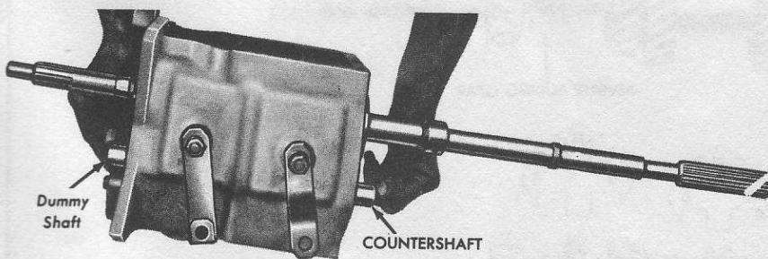
Fig. 6.8 Removing the countershaft (3-speed) (Sec. 3)
