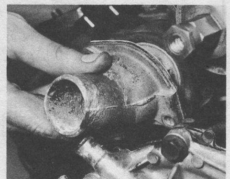
6.4 Removing the thermostat housing
