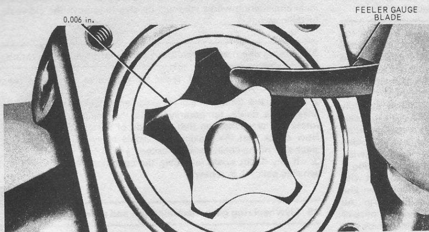
Fig. 1.29 Checking the oil pump inner rotor lobe clearance (Sec. 40)
