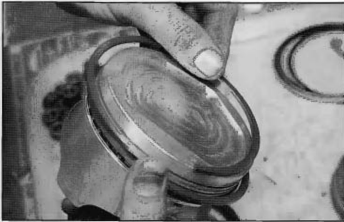
Compression rings are installed next. Locate these end gaps 90 degrees around the piston from the oil-ring gaps.
