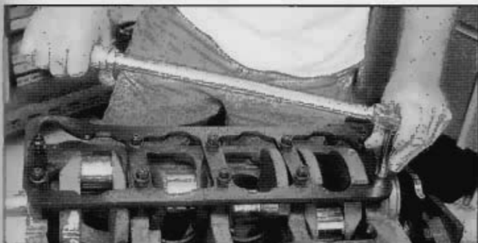
The mains are torqued to specs as shown. Crankshaft end play will be checked next.
