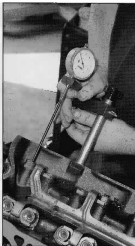
John Da Luz of JMC Motorsports degrees the camshaft and checks crankshaft indexing at the same time. This determines proper camshaft specifications and piston deck height.
