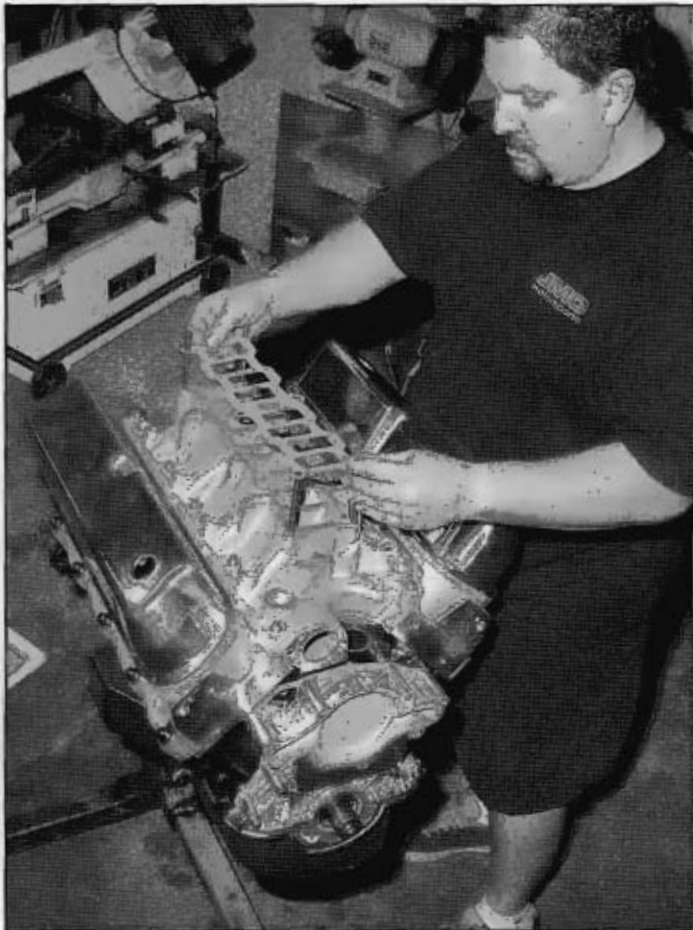
A gasket is placed between the upper and lower intake manifolds.
