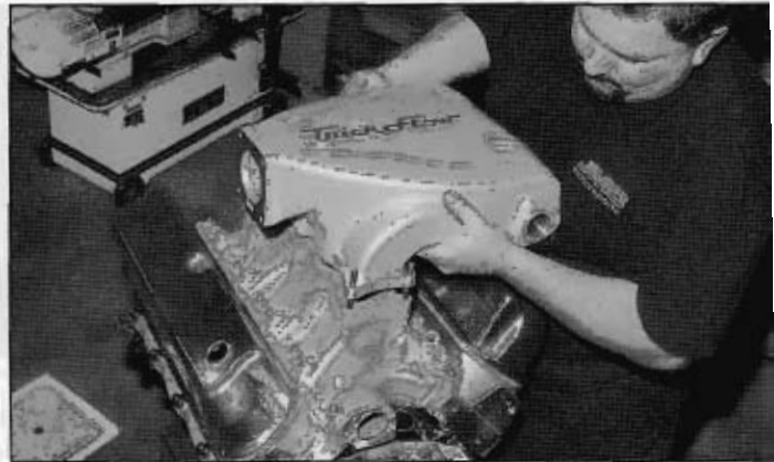
John lowers the Trick Flow upper intake manifold in place.
