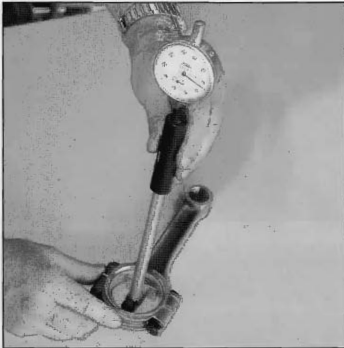
Rod bearing dimensions are checked, as are the crankshaft journals mentioned earlier.
