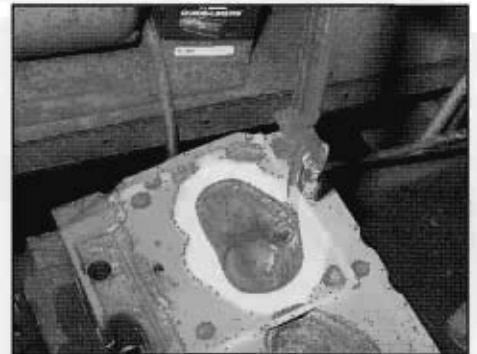
Combustion chamber size is calculated with a graduated scale filled with fluid. Using clear glass over the chamber as shown, using white grease as a seal, we fill the chamber with fluid. When we have completely filled the chamber, we check the amount of fluid used. This tells us chamber volume in cubic-centimeters.
