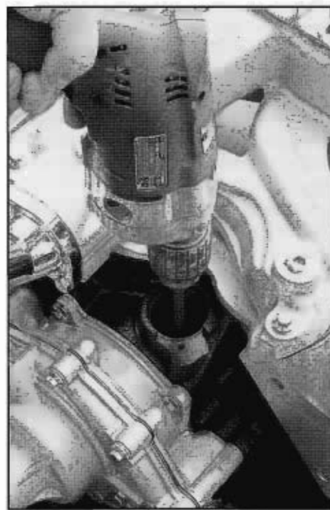
This is an oiling system primer for the small-block Ford. As you can see, it fits into the distributor opening in the block and splines over the oil pump shaft below. You will need a powerful reversible drill for this task.
