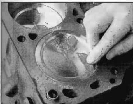
Piston to valve clearance is checked by molding clay into the valve reliefs as shown.
