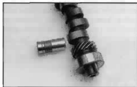
Flat tappets sit on the cam lobe like this. As the cam lobe spins, it spins the lifter in the bore to evenly distribute wear.
