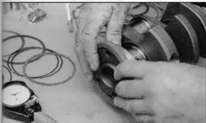
The nice thing about a late-model 5.0L block is the one-piece crankshaft rear-main seal shown here. The one-piece seal provides solid security compared to those old two-piece seals in the 289/302/351W prior to 1982.
