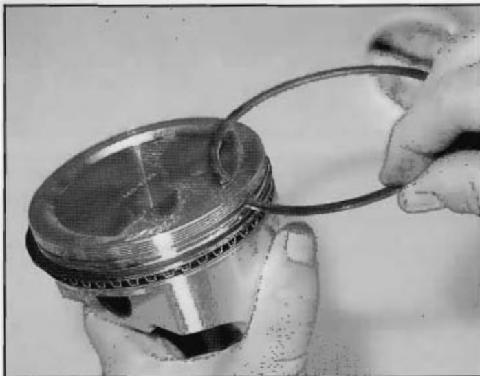
Mark Jeffrey makes piston ring installation look easy. He rolls the compression ring on, doing the second ring first, then the top ring. He stresses always clearing the piston ring lands, making sure you don't nick or scar these critical areas with the ring. Ring gaps must be positioned around the piston in a 9, 12, 3, and 6 o'clock pattern. None of the gaps should be close to one another.
