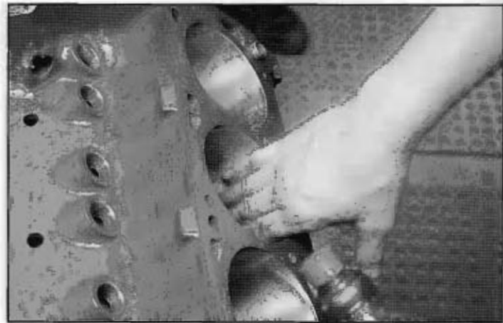
Cylinder walls are wiped clean and lubricated with SAE 30-weight engine oil.
