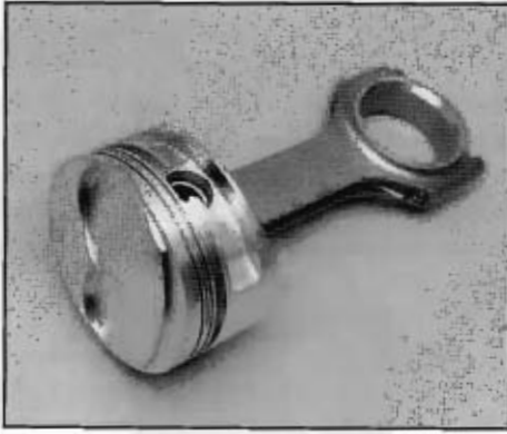
This is a 347ci stroker piston and rod. Note the raised dome (which reduces clearance volume) and the valve reliefs (which increase clearance volume).
