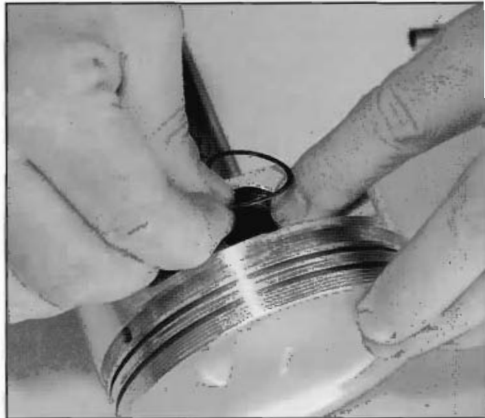
When you build your stroker, expect to see a new kind of piston-pin retaining clip. Instead of the conventional C-clip used for many years, this is a roll-in clip that is easy to install and difficult to remove. The humble C-clip was replaced because they tended to pop out and damage cylinder walls.
