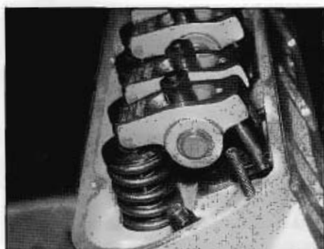
Valvespring installed height looks like this. Always check your spring specs with the retainer installed.
