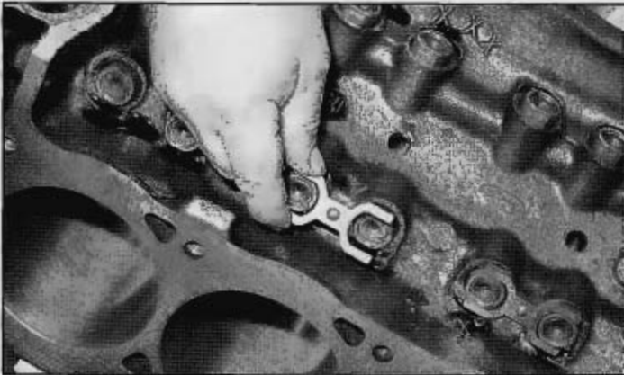
Because this is a roller block, installation is easy. Lifters are seated. Dog bones are installed. And the spider is secured using two bolts screwed into the valley.
