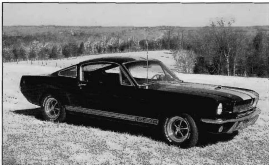
This is a '66 Shelby GT-350H with wide BF Goodrich Radial T/A tires. These tires make an excellent street tire. They offer good handling, coupled with longevity. A softer tire, like the BF Goodrich Comp T/A, holds the road better, but yields less life.
