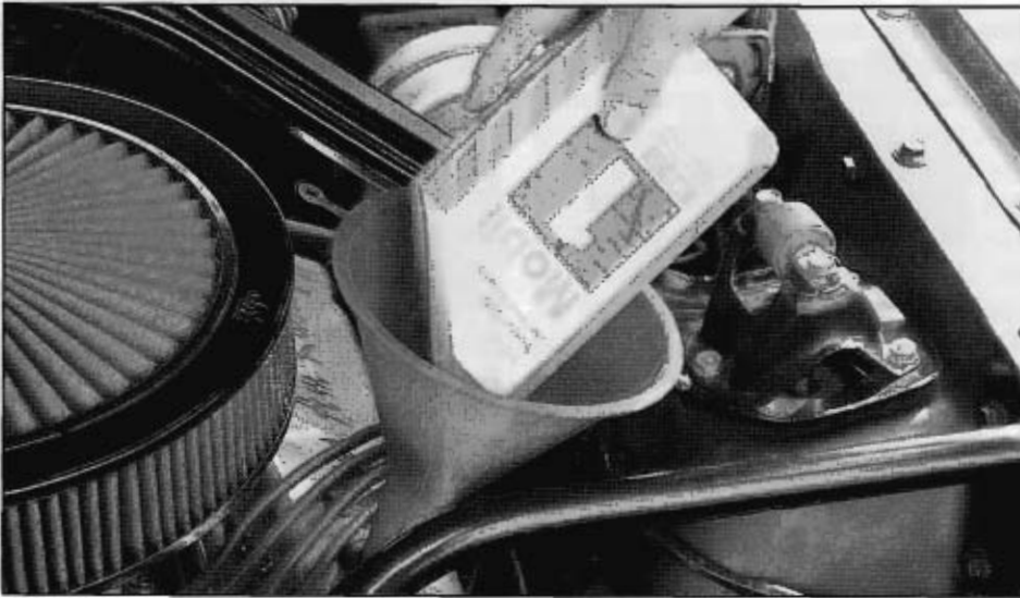
Fill your small-block's oil pan with regular SAE 30 weight engine oil. We suggest the use of Castrol SAE 30 or 10w30 weight oil for your break-in.
