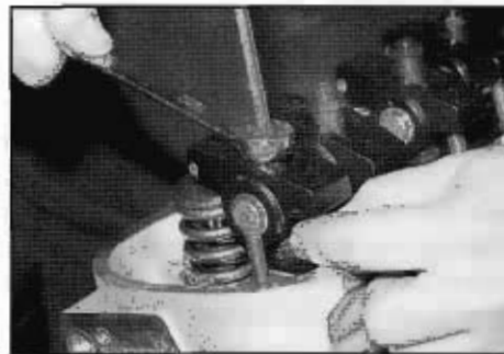
Pushrod length is checked by examining the rocker arm angle as it relates to the valve stem and pushrod.
