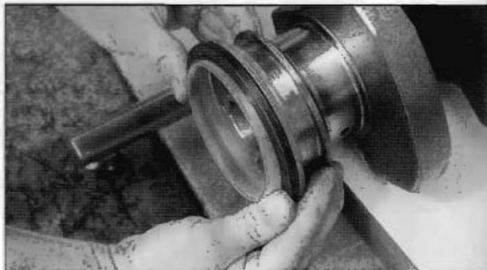
The desirable one-piece rear-main seal has been improved with a plastic installation sleeve, which prevents seal damage or distortion during installation. Mark dresses the crankshaft surface with assembly lube, then slips the seal onto the crank as shown. The plastic sleeve gets tossed.
